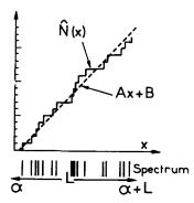
In Ref.[BG-75] a convenient way to compute  $\Delta_{\mathbf{3}}$  (L) has been given, once the ordered sequece of points  $X_1, X_2, \dots, X_n$  in the interval  $[\alpha, \alpha + L]$  is known. Take as origin the center of the interval, i.e., take  $\hat{X}_{1} = X_{1} - (\alpha + \frac{L}{2}); \Delta(L)$ can then be obtained from
