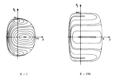
Fig.III.10 - Poincaré maps of the Toda lattice, at energies E = 1 and E = 256 (taken from Ref.[FST-73])
