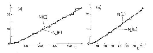
Fig.I.7 - Cumulative density of eigenvalues N(E) of Eq.(I-22) and its average  $N_{KV}$  (E) given by Eq.(I-24) for two different shapes of the boundary : (a) a quarter of a circle of radius unity ; (b) a stadium with straight line and radius of curvature equal to one (See Section IV)(taken from [Sc-84,BGS-84b]).
