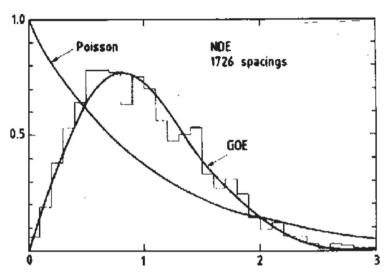
Figure 2. Nearest neighbor spacing distribution for the "Nuclear Data Ensemble" comprising 1726 spacings (histogram) vs. normalized (to the mean) level spacing. The two lines represent predictions of the random matrix GOE ensemble and the Poisson distribution. Taken from Ref. [96]. See also Ref. [71].
