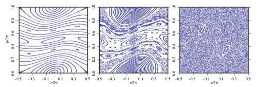
Figure A1. Phase-space portrait (Poincare cross-section) of the kicked rotor for different values of the parameter K. From left to right, K = 0.5, 0.971635, and 5. Images taken from scholarpedia [308].
