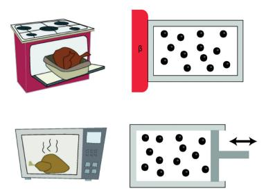
Figure 26. Schematic comparison between the usual thermal heating (traditional oven, top) and an energy increase due to non-adiabatic work (microwave oven, bottom).
