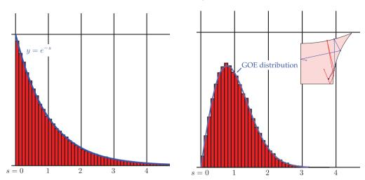
Figure 3. (Left panel) Distribution of 250,000 single-particle energy level spacings in a rectangular two-dimensional box with sides a and b such that  $a/b = \sqrt[4]{5}$  and  $ab = 4\pi$ . (Right panel) Distribution of 50,000 single-particle energy level spacings in a chaotic cavity consisting of two arcs and two line segments (see inset). The solid lines show the Poisson (left panel) and the GOE (right panel) distributions. From Ref. [80].
