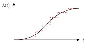
Figure 25. Schematic representation of a continuous process as a series of quenches followed by relaxation to the diagonal ensemble. This approximation is justified if the relevant relaxation time in the system is short compared to the characteristic time scale associated with the change of  $\lambda$ .
