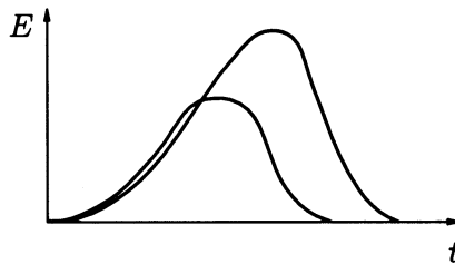
Fig. 2.19. Electric field within a stationary moving domain in AsGa. The domains are moving to the left with the speed 1.2 \times 10^7 \text{ cm s}^{-1} .
