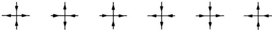
Fig. A.5. The vertices of the two-dimensional ice model which obey the ice rule (two hydrogen atoms near and two more distant)
