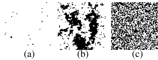
Fig. 5.21 Three snapshots of portions of the Ising model. The Ising model is essentially a lattice of ones and zeros, with white signifying zero and black signifying one. (a) A low temperature T = 1.5 , where all but a few, isolated, random sites are zero. (b) An intermediate temperature, showing some interesting structure. (c) A high temperature, where the pixels are set to zero and one at random. Below: Compressed file sizes, in bits, of the three 256 \times 256 snapshots, using four compression schemes.
