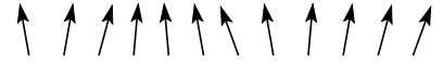
Fig. 9.9 Magnets: spin waves. Magnets break the rotational invariance of space. Because they resist twisting the magnetization locally, but do not resist a uniform twist, they have low-energy spin wave excitations.
