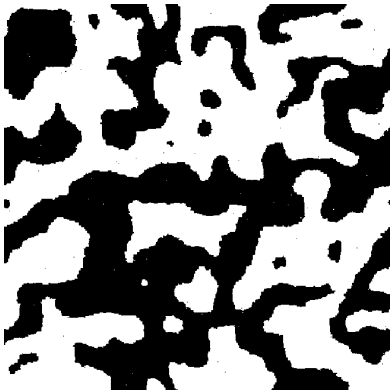
Fig. 10.1 Phase separation in an Ising model, quenched (abruptly cooled) from high temperatures to zero temperature [173]. The model quickly separates into local blobs of up- and down-spins, which grow and merge, coarsening to larger blob sizes (Section 11.4.1).
