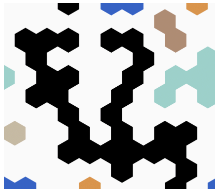
Fig. 2.13 Site percolation network. Each site on a 10 \times 10 triangular lattice is present with probability p = 0.4 , below the percolation threshold for the infinite lattice. Note the periodic boundary conditions at the sides, and the shifted periodic boundaries at the top and bottom.
